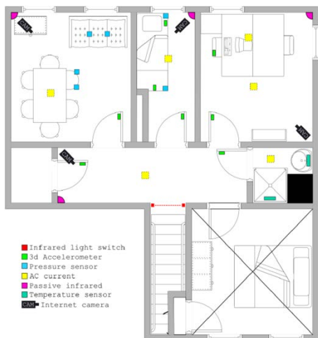
Figure 14. WSN deployment in a home indoor environment (2nd floor) [courtesy: Roessingh Research and Development]
