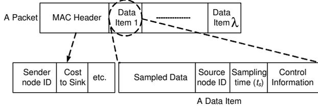
Fig. 2. The structure of a transmission packet in data dissemination.
