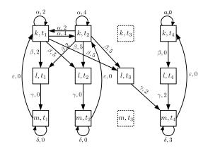
Fig. 2.  $(\max, +)$ -automaton of the example graph.
