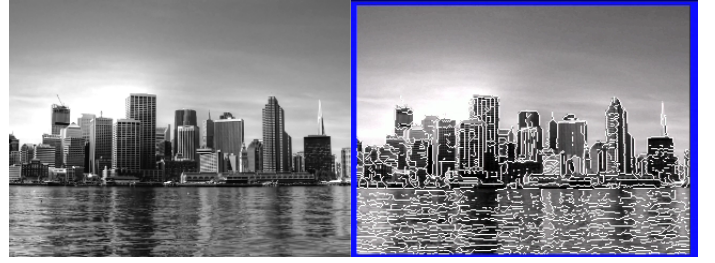
Fig. 14. Original test image (left) and the output of SUSAN. The outer band of the image is skipped.
