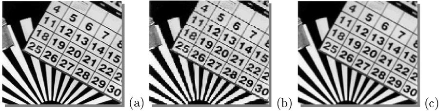
**Figure 1.4:** Photographs of a screen detail showing a comparison of up and down scaling using pixel dropping and repetition, (b), and polyphase-filtering, (c), respectively. The left hand picture, (a) shows the original. Although the result from polyphase filtering is clearly better than that of pixel dropping and repetition, it's resolution is less than that of the original image because of the intermediate scaling to a smaller size.
