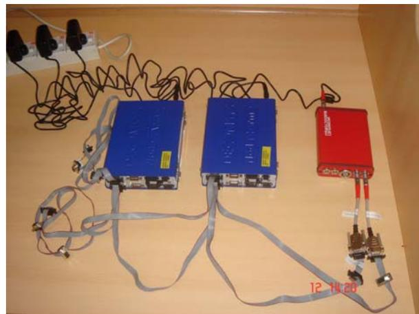
Fig. 7. Overall DECOMSYS setup: ECU (two boxes from left) and Bus Doctor (right most box).
