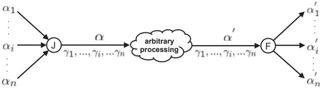
Fig. 3. Join (J) and fork (F) operations on the structured event stream  $\alpha$ . The corresponding ECCs  $\gamma_i$  of sub-streams  $\alpha_i$  remain unaffected after arbitrary processing of the structured event stream  $\alpha$ .
