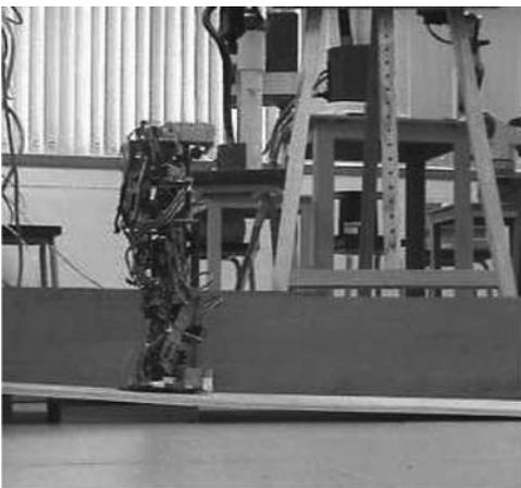
Fig. 20. Walking down a  $3^\circ$  slope.
