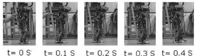
Fig. 17. Robot walking sequence when pushed from behind.
