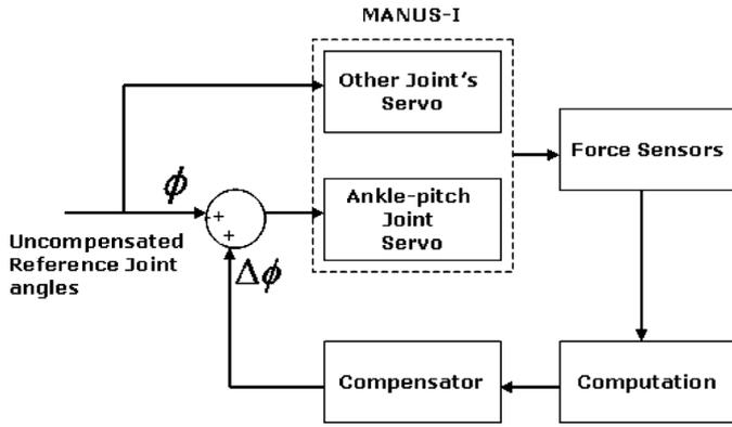
Fig. 9. Block diagram for online ZMP compensation.
