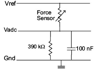
Fig. 5. Force-to-Voltage converter circuit.
