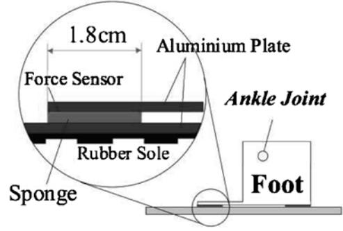
Fig. 4. Mechanical installation of force sensors.
