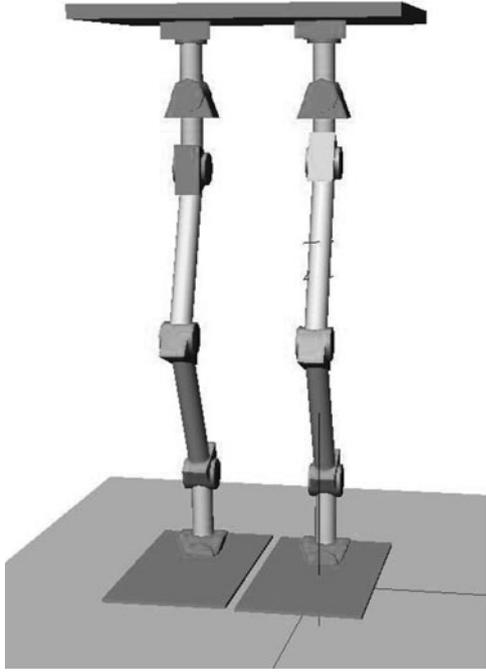
Fig. 2. Biped model of MANUS-I in visualNastran 4D environment.
