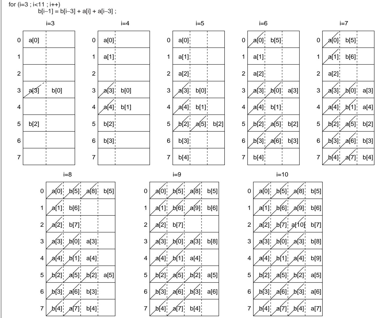
**Figure 8. Initial algorithm and cache states corresponding to different iterations  $i$  of that algorithm for a direct-mapped cache. Diagonal bars represent cache misses. This example has a 100% miss rate: 32/32.**
