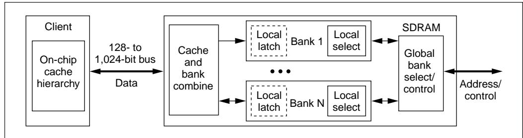
**Figure 10. External data access bottleneck illustration with SDRAM.**
