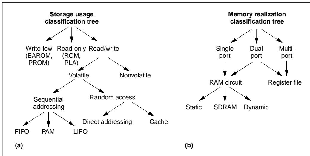
**Figure 2. Storage classification trees: usage (a) and memory realization (b).**
