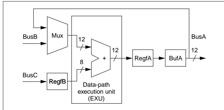
**Figure 1. Register file illustration in a feedback loop of a simple customized data path.**
