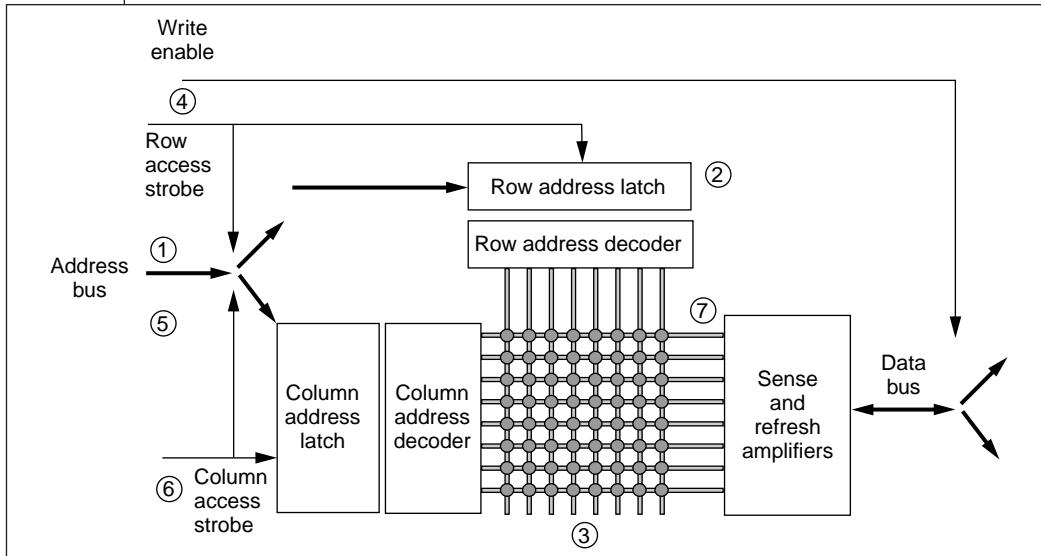
**Figure 9. Illustration of DRAM operation.**
