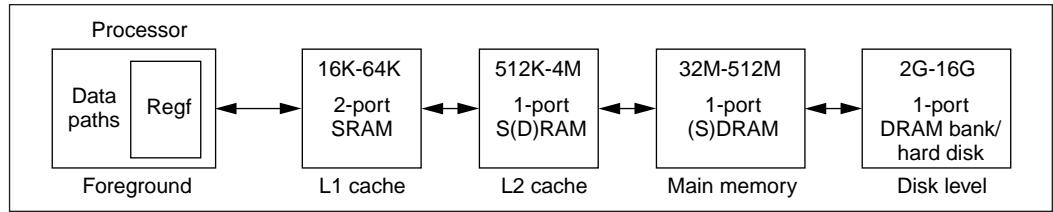
**Figure 3. Hierarchical memory pipeline.**
