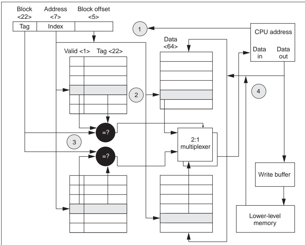
**Figure 6. Eight-Kbyte, two-way associative cache with 32-byte blocks.**
