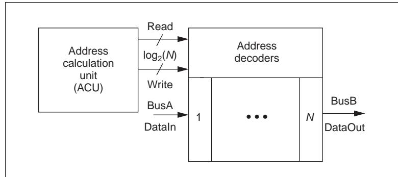
**Figure 4. Two-port register file with a capacity of  $N$  words, with both read and write address supplied in parallel from an address calculation unit.**
