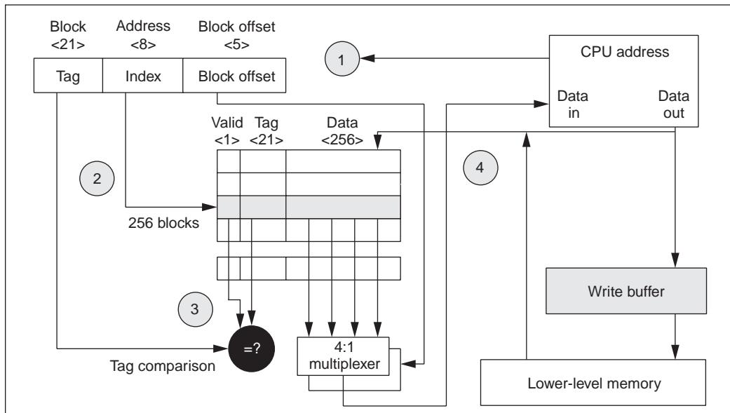
**Figure 5. Eight-Kbyte, direct-mapped cache with 32-byte blocks.**
