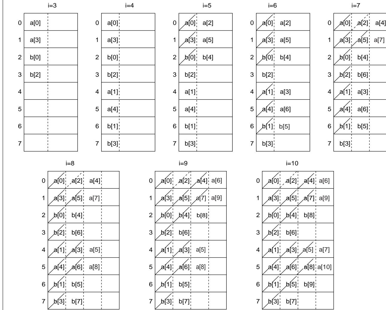
**Figure 7. Initial algorithm and cache states corresponding to different iterations  $i$  of that algorithm for a fully associative cache. Diagonal bars represent cache misses. This example has 26 cache misses: 26/32, an 81% miss rate.**
