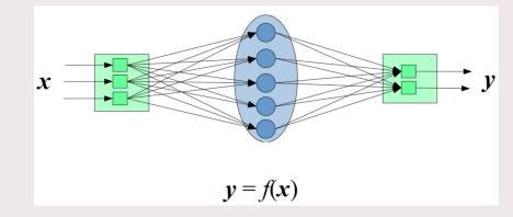
LIF neurons (mean-rate models) Each neuron has its unique tuning curve Given enough neurons we can approximate any functions
