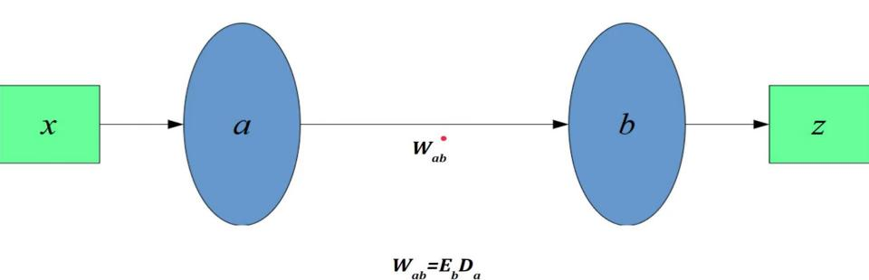
We can generate a set of connections weights by generating two neural networks and then merge them together.
