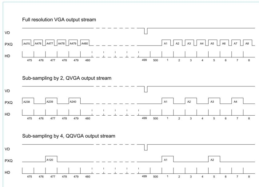
$^{\star}$  Above timing diagrams depict 2 and 4 times sub-sampling. 3 and 5 times subsampling is done in a  $\,$  comparable way.
