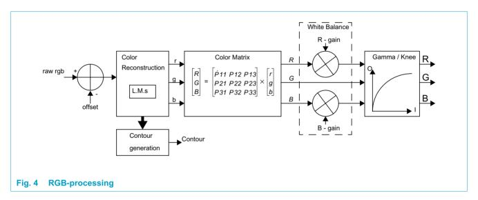
First the input black level is restored to have the data referred to digital code "0". Then the raw RGB signal is applied to a reconstruction function. This function basically generates a triplet of raw RGB data for every pixel of the video stream. Red, green and blue information are recovered for every single pixel by means of spatial filtering, using the physically surrounding colored pixels.
