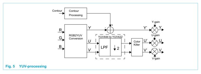
After RGB processing the channels are separated into a luminance (Y) and two color difference paths (UV). The signals are generated using the following formulas:
