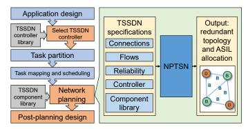
Fig. 1: Design flow of in-vehicle TSSDN
