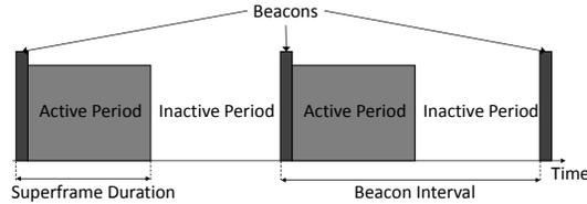
Fig. 3. Time-domain structure of beacon-enabled IEEE 802.15.4
