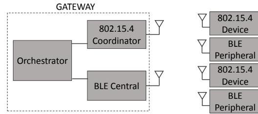
Fig. 4. Network structure for cooperative coexistence solution
