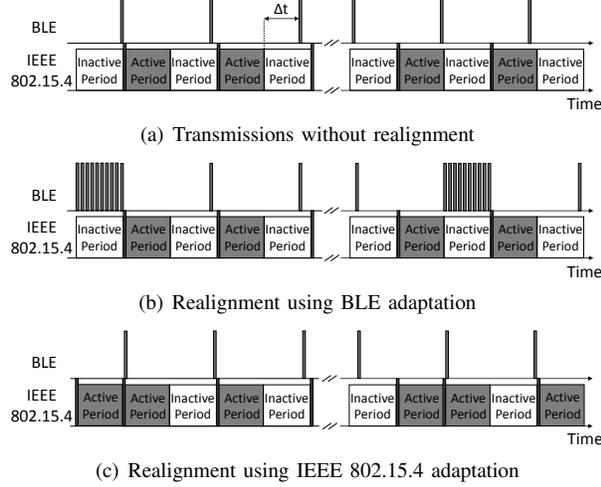
Fig. 7. BLE and IEEE 802.15.4 transmissions without and with realignments for  $BI > CI$
