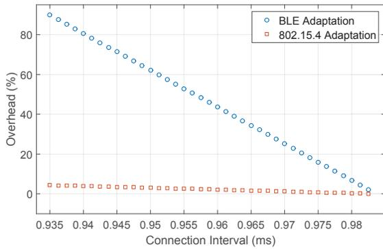
Fig. 11. Overhead of the algorithms for  $BO = 6$  and  $SO = 5$
