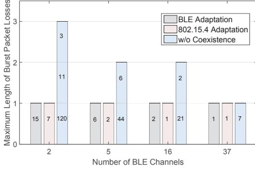
Fig. 9. Maximum length of burst and the number of losses for each length of burst for 1000 transmission attempts on a BLE link
