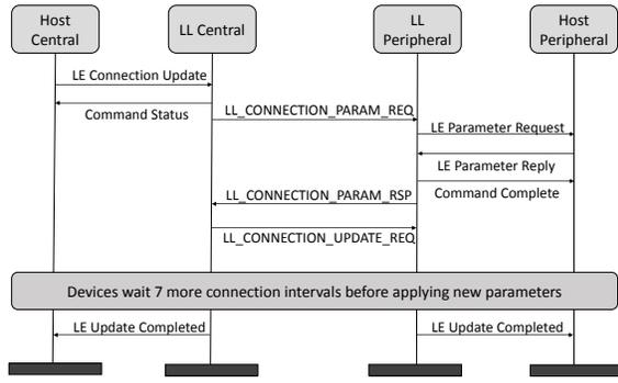
Fig. 6. The message sequence required for a BLE CI update
