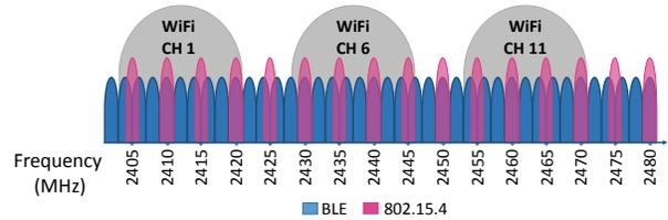
Fig. 1. Channels of BLE, IEEE 802.15.4, and WiFi in 2.4 GHz
