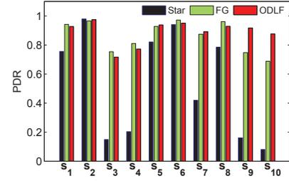
Fig. 9. PDR of different body sensor nodes to the gateway in an experiment with low quality links.
