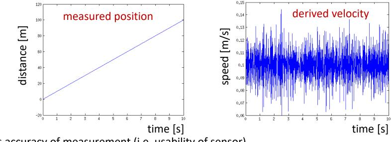
noise limits accuracy of measurement (i.e. usability of sensor)
