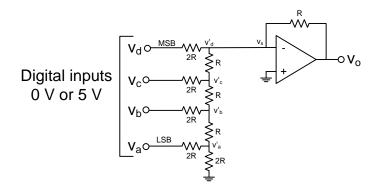
Figure 3: DA converter using ladder network.
