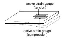
Figure 1: Metal strip with two active strain gauges.
