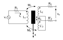
Figure 4: LVDT sensor.
