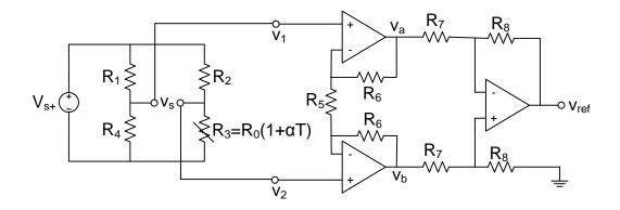
Figure 6: Implementation of "RTD-based sensor" block of Figure 5.
