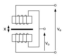
Figure 4: Inductive sensor based on two coils in series.
