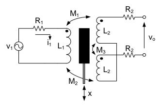
Figure 5: LVDT sensor.
