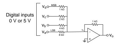
Figure 8: DA converter using summing op-amp.
