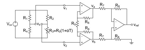
Figure 2: Implementation of "RTD-based sensor" block of Figure 1.
