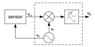
Figure 6: Sensor with phase sensitive detector.
