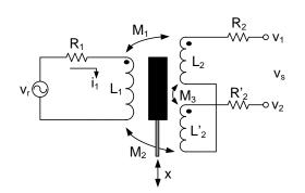
Figure 4: Measuring a displacement using an LVDT.
