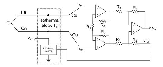
Figure 1: Compensation with a RTD-based sensor and instrumentation amplifier.
