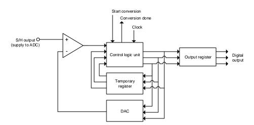
Figure 7: Successive approximation AD converter.
