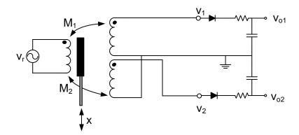
Figure 5: Double-sided rectifier with low-pass filter.
