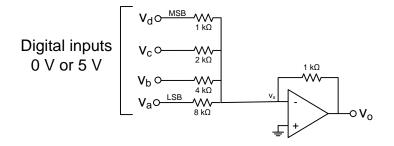
Figure 2: DA converter using summing op-amp.
