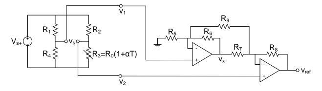
Figure 6: Implementation of "RTD-based sensor" block of Figure 5.
