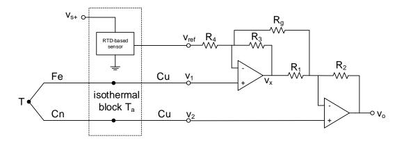
Figure 5: Compensation with a RTD-based sensor and instrumentation amplifier.
