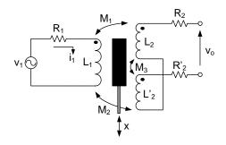
Figure 3: LVDT sensor.
