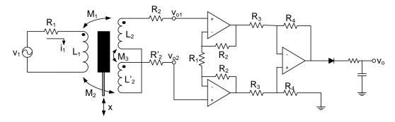
Figure 4: Single-sided rectifier with low-pass filter.
