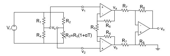
Figure 7: Sensor circuit connected to instrumentation amplifier.
