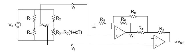
Figure 2: Implementation of "RTD-based sensor" block of Figure 1.
