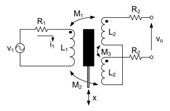
Figure 4: LVDT sensor.
