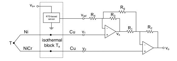
Figure 1: Compensation with a RTD-based sensor and instrumentation amplifier.
