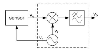
Figure 5: Sensor with phase sensitive detector.
