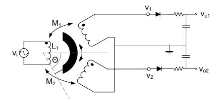
Figure 5: Double-sided rectifier with low-pass filter.
