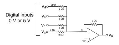
Figure 9: DA converter using summing op-amp.
