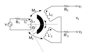
Figure 4: Measuring an angle using an RVDT.
