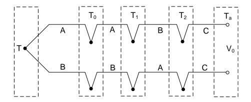
Figure 8: Simulate reference junction at 0°C.
