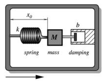
Figure 1: Mechanical model of an acceleration sensor.
