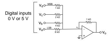
Figure 3: DA converter using summing op-amp.
