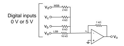
Figure 4: Alternative DA converter.
