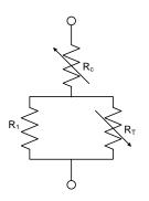
Figure 3: Temperature compensation using an NTC thermistor.
