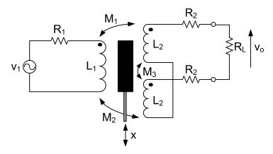
Figure 2: LVDT sensor.
