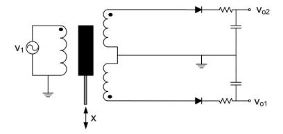
Figure 4: Double-sided rectifier with low-pass filter.
