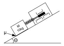
Figure 1: Meausing inclination using an LVDT.
