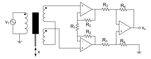
Figure 2: Amplification of the LVDT output signal.
