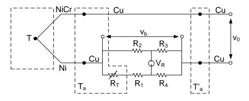
Figure 1: Circuit for cold junction compensation.
