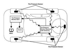
Figure 1: Tire-pressure monitoring system.
