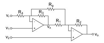
Figure 3: Instrumentation amplifier with two op-amps.
