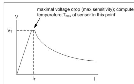
(The temperature  $T_{max}$  is the temperature which the sensor reaches at the point iin which the voltage drop across  $V_T$  the sensor is maximal. Note that this is not the maximal temperature which the sensor can reach. This temperature is much higher. If you increase the current I further, the self-heating effect will continue to increase and therefore also T.)
