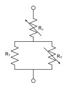
Figure 3: Temperature compensation using an NTC thermistor.
