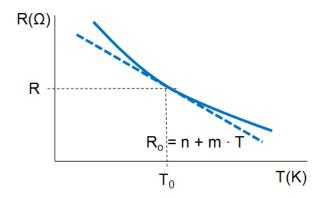
Since it is required that the transfer function shows an inflection point at  $T_0$ , it must hold that the second derivative of R to T is equal to 0 in this point  $(T_0)$ . The first derivative is equal to:
