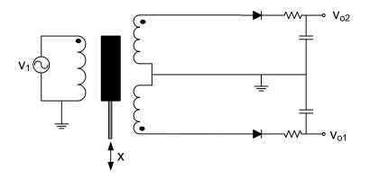
Figure 4: Double-sided rectifier with low-pass filter.
