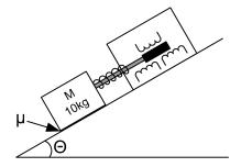
Figure 1: Meausing inclination using an LVDT.
