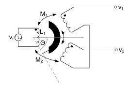
Figure 1: Measuring an angle using an RVDT.
