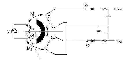
Figure 4: Double-sided rectifier with low-pass filter.
