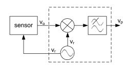
Figure 3: Sensor with phase sensitive detector.
