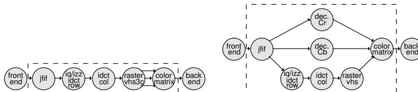
Figure 9: JPEG decoder (Design 5 and Design 6).
