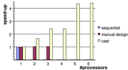
Figure 13: Speed-up of 3DRS implementations.
