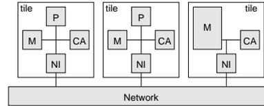
Figure 1. MP-SoC architecture template.
