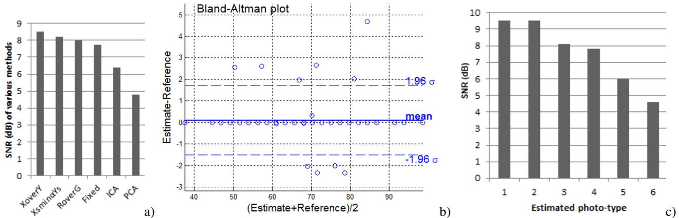
Fig. 7. a): The obtained SNR for the various methods obtained from our database of 117 static persons. b): Bland-Altman plot indicating 92% good agreement ( $\pm 1.96\sigma$ ) between rPPG and contact PPG (shown for *XoverY* method). c): The SNR as a function of the estimated photo-type shows that increased melanin content of the skin leads to a reduced fraction of the diffusely reflected light from the skin and consequently a decreased SNR of the rPPG signal.
