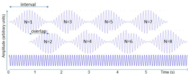
Fig. 5. Illustration of the overlap-add procedure. Every interval an optimized pulse-signal is calculated and multiplied with a Hanning window. Half the interval length later this is repeated and the pulse output signal (bottom) results as the sum of these overlapping pieces.
