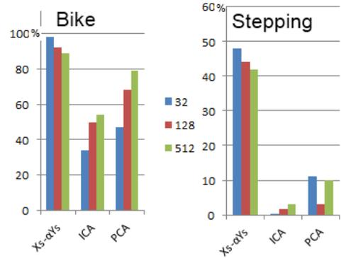
Fig. 6. Percentage of time that the frequency peak corresponds to pulse-rate for overlap-add interval of 32 up to 512. The chrominance-based methods perform better for shorter intervals. Methods based on BSS, however perform best with longer intervals. With serious motion (stepping device), this may be the reason BSS-based methods break down completely.
