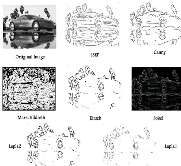
Figure 2: Edge detection results, derived for Car Image
