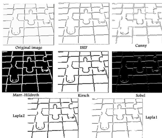
Figure 1: Edge detection results, derived for Chess Image
