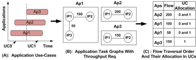
Fig. 3. Application Flow Traversal Order And UC Allocation
