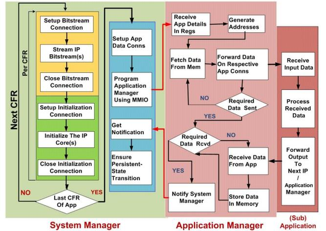
Fig. 4. Loading An Application
