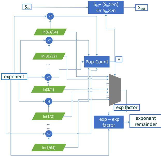
Fig. 3: Simplified RTL of first stage of Logarithmic scaling.
