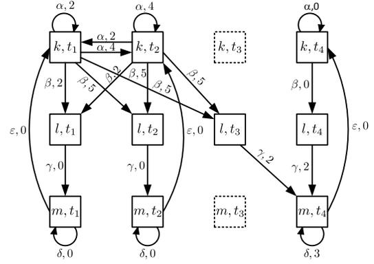
Fig. 2.  $(\max, +)$ -automaton of the example graph.
