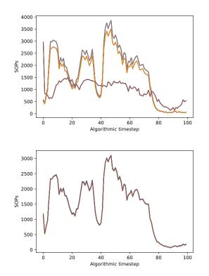
Fig. 7: SOPs performed by each tile for 4x4 mesh mappings with different layers separated (top) and merged together (bottom). Merging layers balances SOP load. 4x4 mappings perform less SOPs per tile compared to 3x3 mappings.
