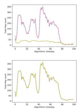
Fig. 6: Spike hops passing through each tile for 3x3 mesh mapping with different layers separated (top) and with different layers merged together (bottom). Merging hidden layers together on all cores results in increased communication.
