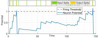
Fig. 1: The response of an LIF neuron (bottom) to incoming random spikes (top). The LIF neuron potential leaks exponentially in time and it fires when it crosses firing threshold.
