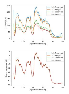
Fig. 9: Latency (top) and energy (bottom) estimates per algorithmic timestep for MorphIC model. We notice performance is overwhelmingly dominated by SOPs and not spike hops.
