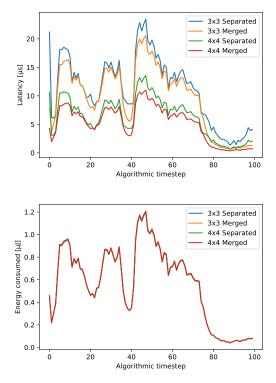
Fig. 10: Latency (top) and energy (bottom) estimates per algorithmic timestep for Loihi model.
