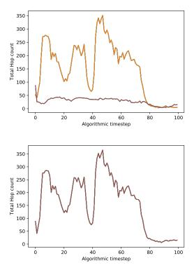
Fig. 8: Spikes routed by each tile for 4x4 mesh mappings with different layers separated (top) and merged together (bottom). Merging layers together on cores increases spike traffic. 4x4 mappings have more spike traffic compared to 3x3 mappings.
