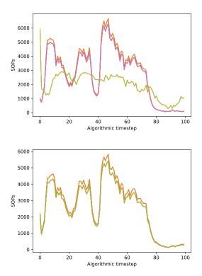
Fig. 5: Synaptic operations performed by each tile for 3x3 mesh mapping with different layers separated (top) and with different layers merged together (bottom). Merging hidden layers together on all cores results in more balanced SOP load.
