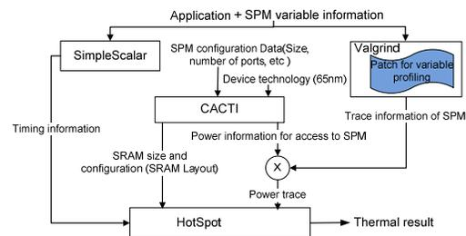
Fig. 5. Tool flow for thermal simulation
