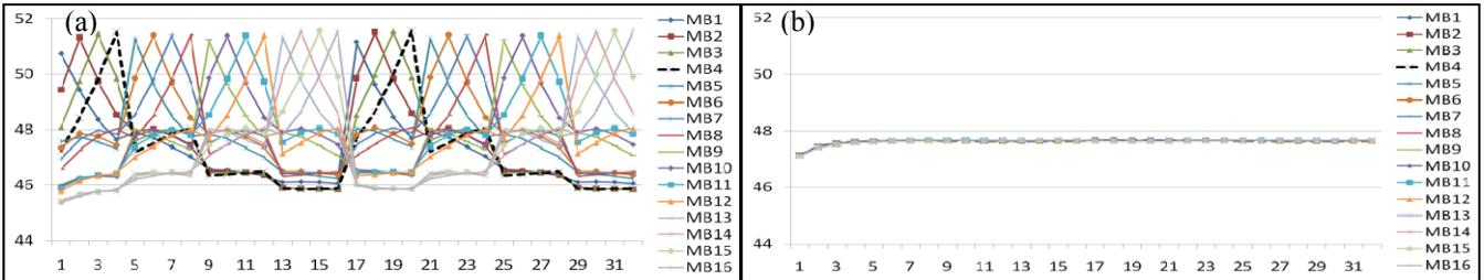
Fig. 7. Motion estimation-SPM surrounded by inactive silicon, average temperature ( $^{\circ}\text{C}$ ) of memory bank (vertical axis) versus time period (horizontal axis). (a) temperature result for baseline solution (b) temperature result for address mirroring technique.
