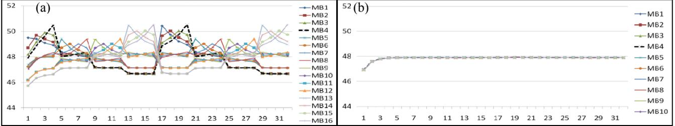
Fig. 8. SUSAN-SPM surrounded by air, average temperature ( $^{\circ}\text{C}$ ) of memory bank (vertical axis) versus time period (horizontal axis). (a) temperature result for baseline solution (b) temperature result for address mirroring technique.
