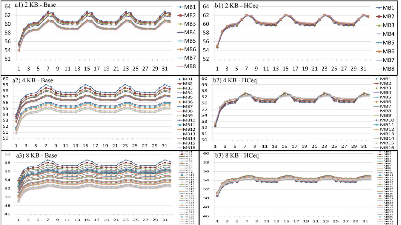
Fig. 9. MP3 decoder-SPM surrounded by air, average temperature ( $^{\circ}\text{C}$ ) of memory bank (vertical axis) versus time period (horizontal axis). (ax) temperature result for baseline solution (bx) temperature result for HCEq technique.
