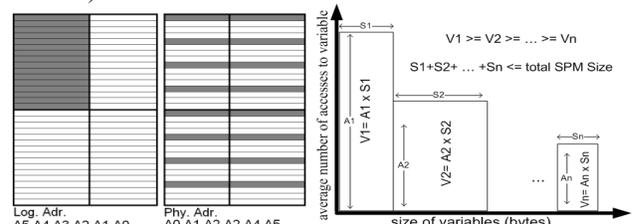
Fig. 3. Logical to physical address mapping.
