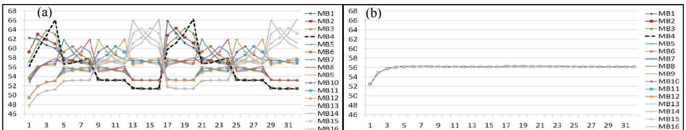
Fig. 6. Motion estimation-SPM surrounded by air, average temperature (°C) of memory bank (vertical axis) versus time period (horizontal axis). (a) temperature result for baseline solution (b) temperature result for address mirroring technique.
