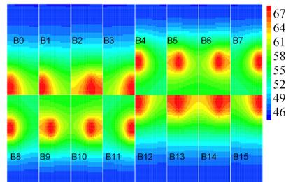
Fig. 1. Temperature of SPM while running the motion estimation application.
