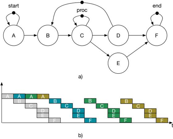
Fig. 4. Example with natural static-order between actors B and D
