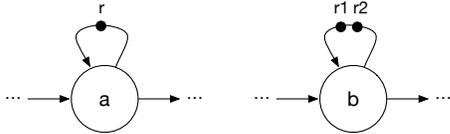
Fig. 10. Modeling resource binding in actors: (a) actor  $a$  is bound to resource  $r$  (b) actor  $b$  is bound two resource  $r$  with a capacity of 2
