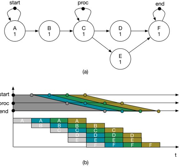
Fig. 2. (a) Example application graph modeled as an SDFG graph (b) Gantt chart execution of 4 iterations of the example application
