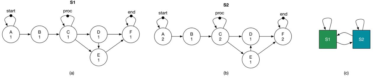
Fig. 1. Example FSM-SADF application graph: (a) Scenario S1 (b) Scenario S2 and (c) Finite-State Machine that models scenario flow
