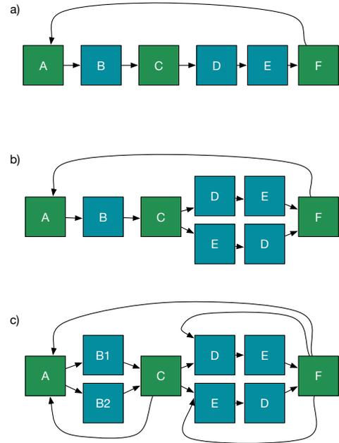
Fig. 7. FSM representing different stages of the modeling: a) Application flow with set bindings and actor order, b) Resource-Sharing (Orderings) and c) Resource Binding
