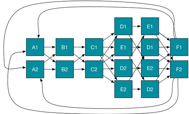
Fig. 11. FSM that holds all the behavior of our example application mapped on a 2-Homogenous resource platform
