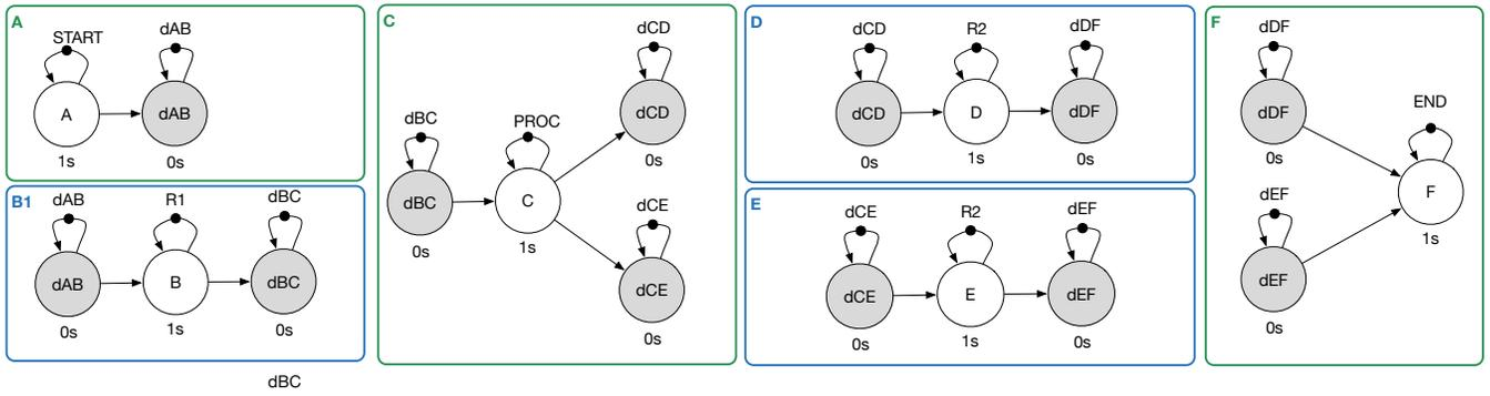
Fig. 8. Adaptation of the splitting of the SDFG of Fig. 6 into scenarios of the SADf model
