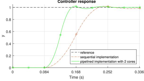
Figure 2: Controller response of motivational example with and without pipeline. The round markers denote multiples of the sampling period.
