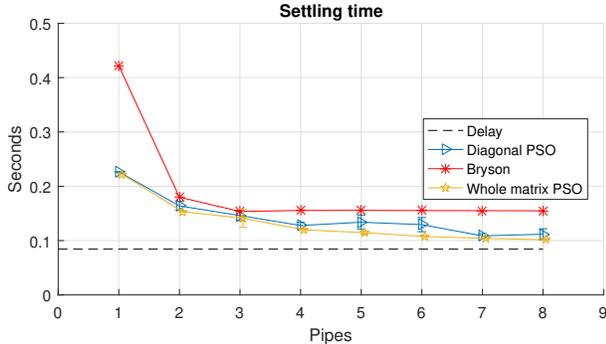
Figure 3: Tuning of LQR with different approaches.
