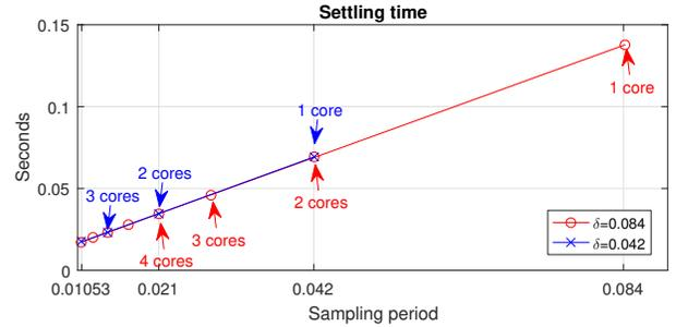
Figure 6: Impact of sampling period on settling time (with sensing delay subtracted for comparison purposes).
